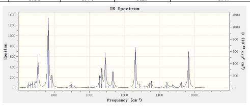
**Figure S1.** The theoretical FTIR spectrum of optimized oligo-Py molecule containing 6 units calculated by B3LYP/6-31+G(d) method with gaussian09 software.
