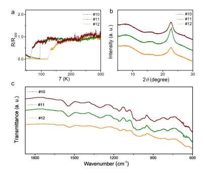
**Figure S3.** The performance of the PPy samples with superconducting-like property. The samples (#10-12) were fabricated using paper as substrates, FeCl<sub>3</sub> as oxidant (1 M). (a) The relationship between resistance and temperature from 50 to 300 K. (b,c) The XRD patterns and the FTIR spectra of the three PPy samples.
