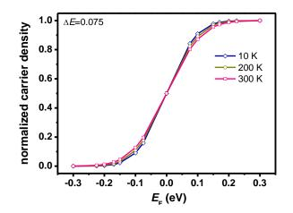
Figure S2. The relation between the carrier densities and  $E_F$  at different temperature with  $\Delta E = 0.075$  eV.
