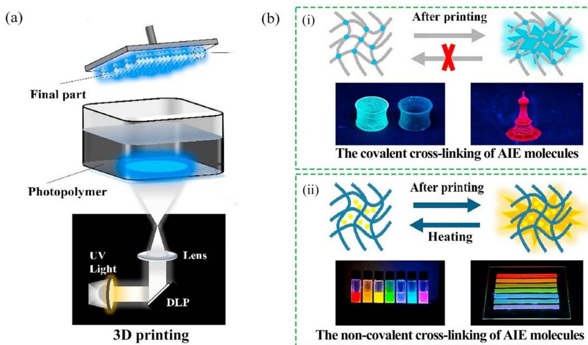
**Figure 2.** DLP printing studies of AIE polymers. (a) Illustration of the top-down printing process in the DLP 3D apparatus. (b) Two different fluorescence mechanism maps of covalent and non-covalent interactions of AIE molecules (i) AIE molecular covalently cross-linked thermosetting photocuring resin, (ii) AIE molecules are doped into thermoplastic photocurable resins, and multi-color 3D printing. Reprinted from [7], © 2020 Published by Elsevier Ltd.
