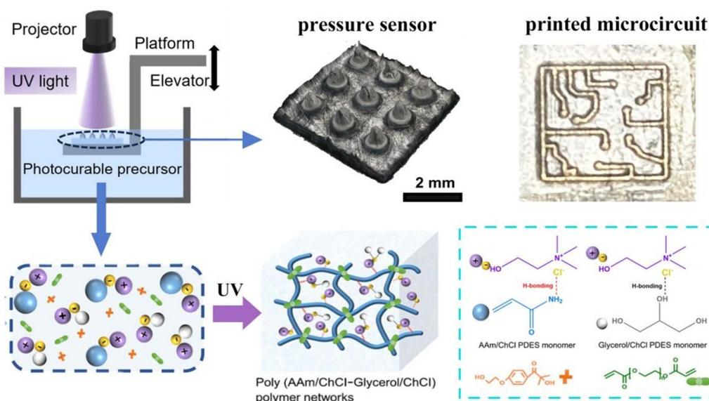
**Figure 5.** 3D printing of self-healing, degradable, conductive ionic elastomers based on polymerizable deep eutectic solvents. Reprinted from [96], © 2024 Elsevier B.V. All rights reserved.
