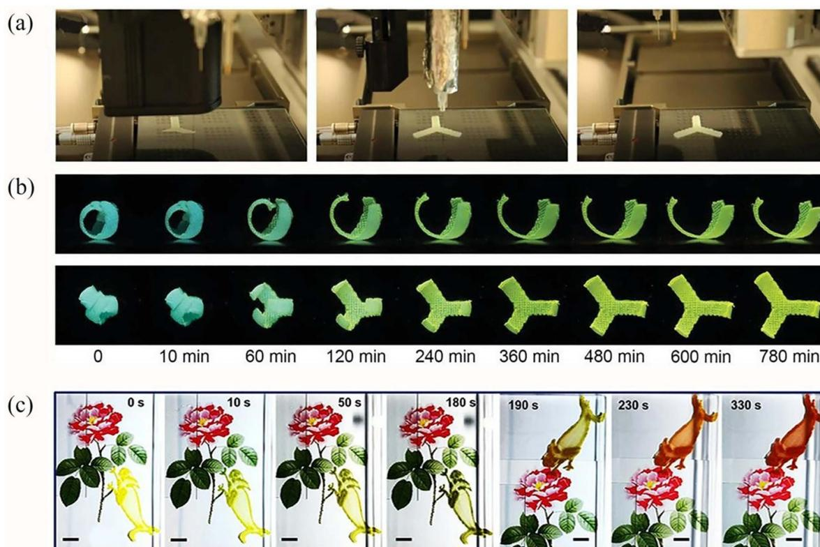
**Figure 8.** 3D printing of AIE materials for 4D print. (a) The 3D printing process of the three-arm actuator. (b) The fluorescent-color-fluorescent-luminescence-shape response of the three-arm actuator. (a), (b) [73] John Wiley & Sons. © 2020 WILEY-VCH Verlag GmbH & Co. KGaA, Weinheim. (c) The continuous discoloration process of the PLA-CMVMN chameleon sensor at different time intervals (0–180 s: diethylamine vapor, 190–330 s: n-butylamine vapor). Reproduced from [76]. CC BY 4.0.
